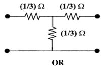
Determine the Z parameters of the following two-port network. 10M
